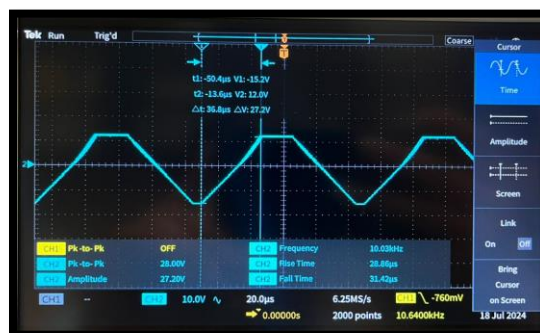
Figure 21.- Non-Inverting Amplifier showing a finite rise/fall time with a square wave.
