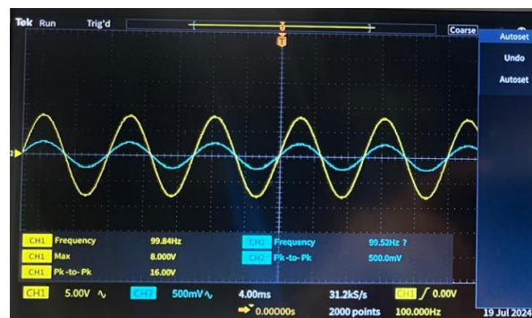
Figure 22.- Non-Inverting Amplifier showing a sine wave at 100Hz.
